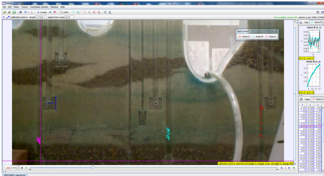
Figure 4: Collecting Well Head Data via Tracker
