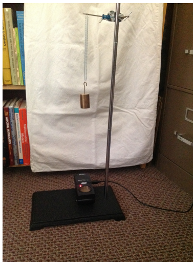
Figure 3. The apparatus for collecting data on the bouncing spring mass system with the VernierGo!Motion Detector on the floor. The spring was pulled down and released and the detector collected data on the changing distance between the mass and the collection head of the detector.
