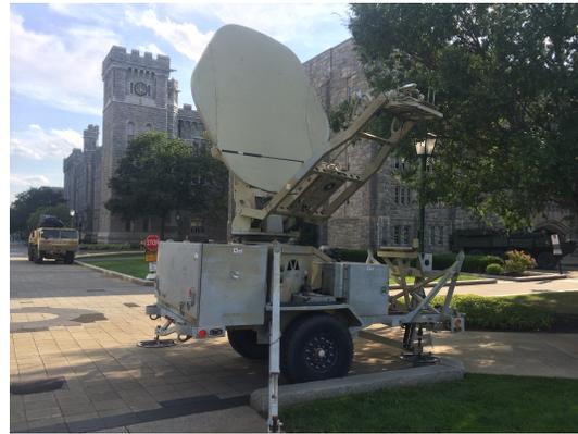
These rugged, trailer-based earth terminals deliver up to 56 Mbps (mega bytes per second) throughput - and they can be towed anywhere a HMMWV (High Mobility Multipurpose Wheeled Vehicle) can go. Rockwell Collins has built more than 800 STT units since the JNN program's inception in 2004. [Rockwell Collins 2009] Due to recent budget cuts, more economical parts must be used in the production of STTs. Engineers have tasked you with comparing feasible options for the suspension systems of the STTs.
